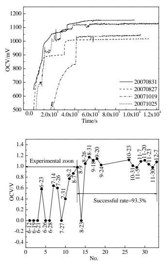
Fig.3 The successful rate for the OCV of more than 1V
