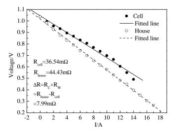
Fig.6 Resistance measurement of electrical current leads and contacts
