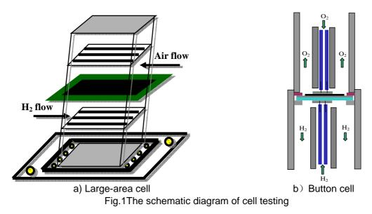
Fig.1a) shows the schematic diagram of testing for large-area cell, and b) for button cell. The technique of testing for button cell is widely used due to the application of ceramic tube
