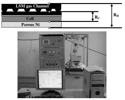
Fig.5 Set-up of cell testing for large-scale planar SOFCs
