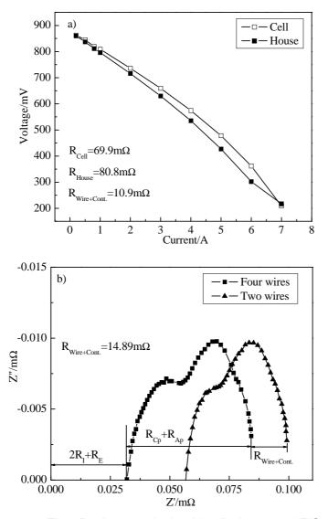
Fig.7 Resistance obtained by discharge and EIS
