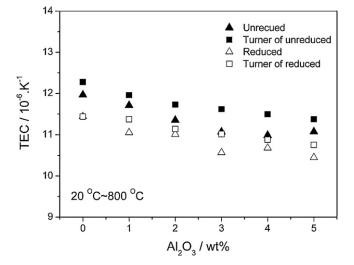
**Fig. 6.** Comparison of the measured TECs with those calculated by Turner's equation as a function of alumina content before and after reduction.
