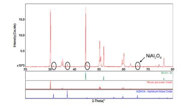
Fig. 4. XRD patterns of sintered anode support material (Ni-YSZ)<sub>0.95</sub>(Al<sub>2</sub>O<sub>3</sub>)<sub>0.05</sub>.
