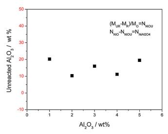
**Fig. 5.** The content of unreduced alumina in the anode support material  $(NiO-YSZ)_{1-x}(Al_2O_3)_x$  as a function of total alumina content.
