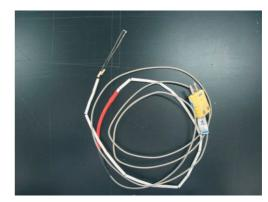
Fig. 3 The thin-K type thermocouple.
