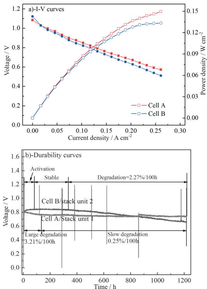
Fig. 4 I-V curves and durability curves of stack 2: (a) I-V curves and (b) durability curves.
