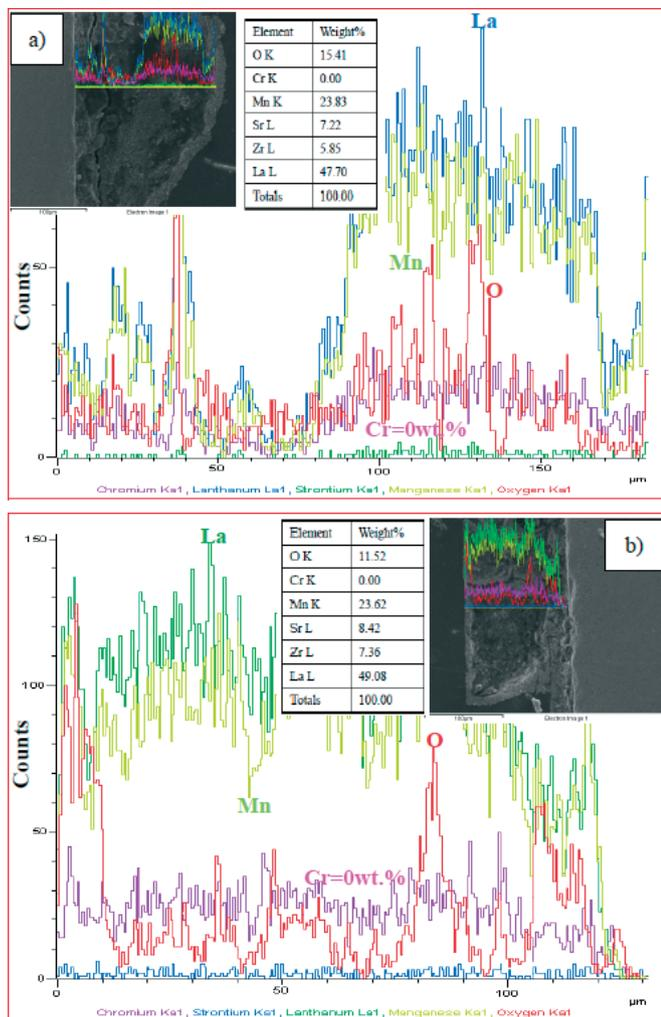
Fig. 14 EDS line in cell cathode: (a) cell A and (b) cell B.
