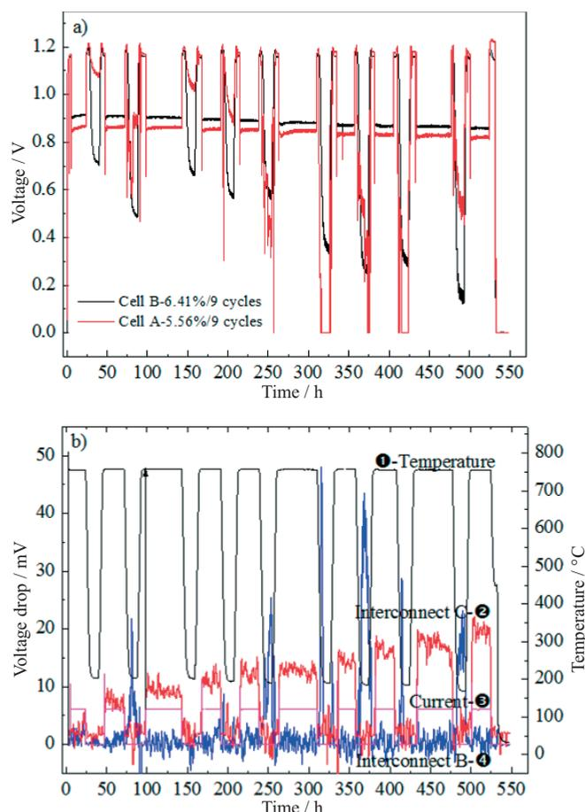
Fig. 12 Cell degradation and voltage drop caused by interconnect under thermal cycles: (a) cell degradation and (b) voltage drop curves caused by uncoated interconnect B-curve ④ and by coated interconnect C-curve ②, current – curve ③, and temperature – curve ①.
