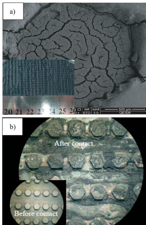
Fig. 15 Contact traces on cathode side of cell A and uncoated interconnect B: (a) cathode side of cell A and (b) cathode side of interconnect B.
