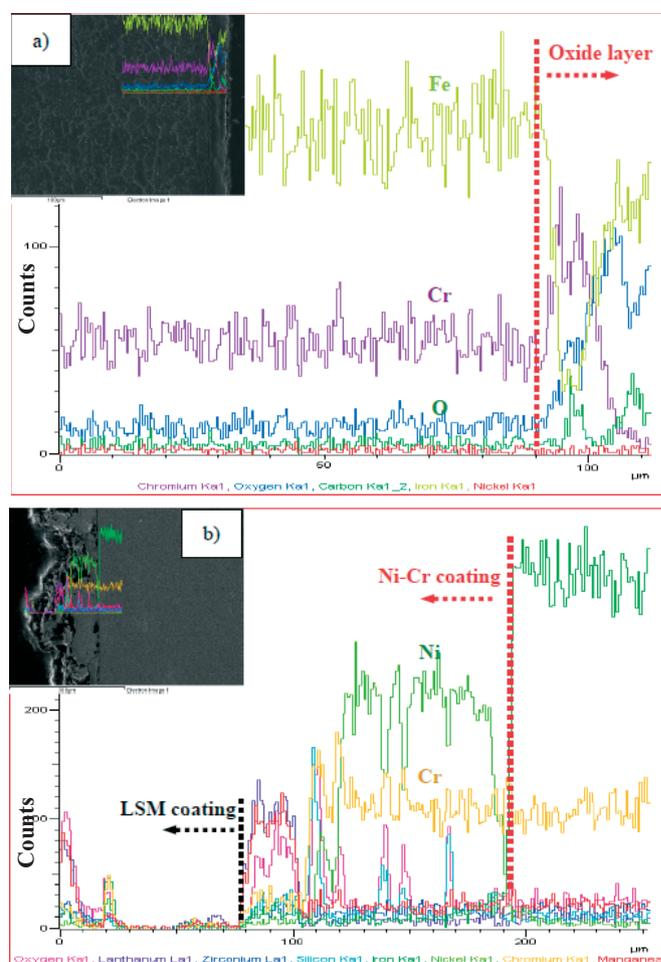
Fig. 13 EDS line on cathode side of interconnect: (a) uncoated interconnect B and (b) coated interconnect C.
