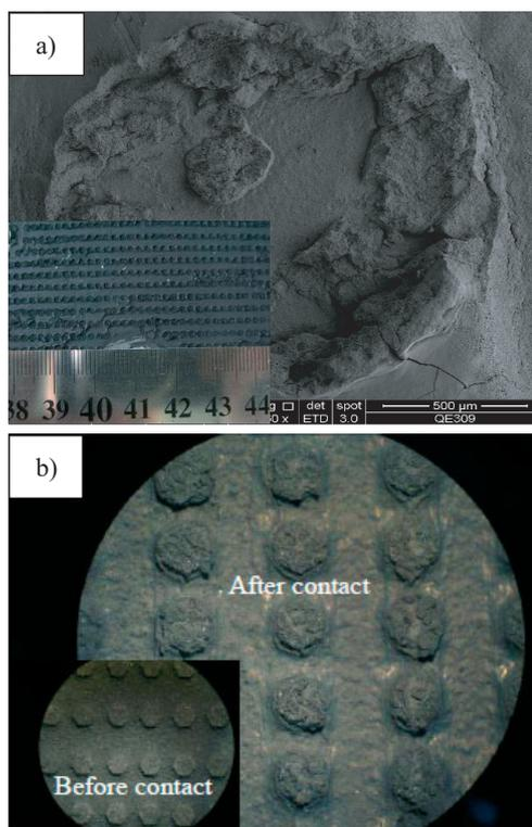
Fig. 16 Contact traces on cathode side of cell B and coated interconnect C: (a) cathode side of cell B and (b) cathode side of interconnect C.
