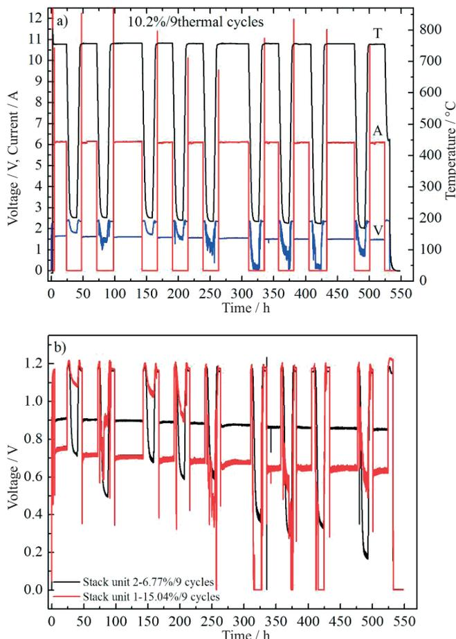
Fig. 11 Degradation of stack and its stack unit under thermal cycles: (a) stack and (b) stack unit.
