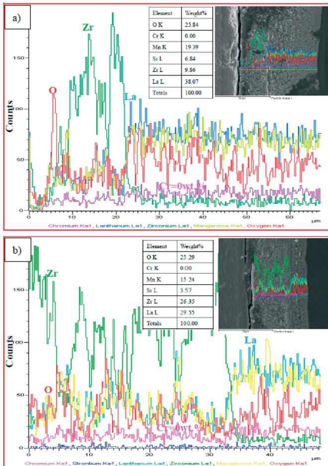
Fig. 7 The morphology and EDS line of cell: (a) cell A and (b) cell B.
