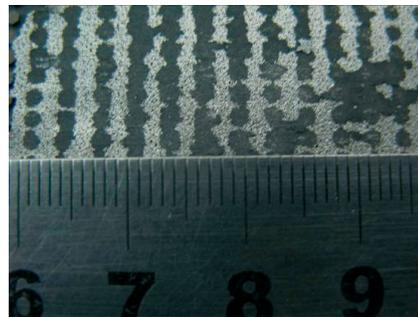
Fig. 8 Contact traces on cell anode sides after testing in stack 1 and stack 2.
