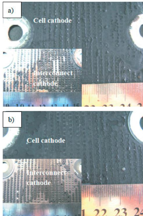
Fig. 9 Contact traces on cell cathode sides after testing in stack 1: (a) cathode side of cell A and interconnect B, and (b) cathode side of cell B and interconnect C.
