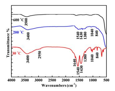
Fig. 4. FT-IR spectra of GDC precursors heat-treated at 30, 200 and 600 °C (L/M=0.5).
