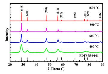
Fig. 3. XRD patterns of GDC powders calcined at 400, 600, 800 and 1500 °C, respectively (L/M=0.5).
