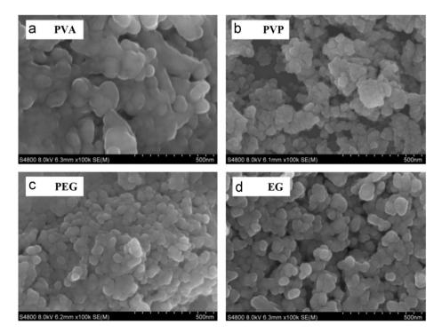
Fig. 7. SEM photographs of the GDC powders calcined at 600 °C with different surfactants (a) EG, (b) PEG, (c) PVA and (d) PVP (L/M=0.5).
