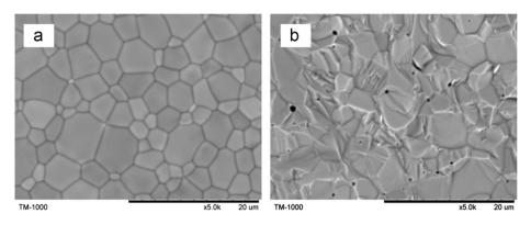
Fig. 8. SEM photographs of the surface (a) and fracture surface (b) of GDC pellet calcined at 1500 °C.
