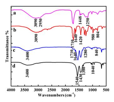
Fig. 6. FT-IR spectra of: (a) PAA, (b) AA, (c) AA and cerium and gadolinium acetates and (d) cerium and gadolinium acetates (molar ratio of acrylic acid to metallic ions is 0.5 and the ratio of cerium acetates to gadolinium acetates is stoichiometric).
