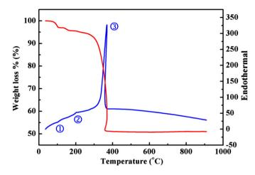
Fig. 2. TG/DTA curves of GDC precursor dried at 30 °C.
