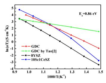
Fig. 9. Arrhenius plot of ionic conductivity of GDC,GDC in Tao [2], SSZ and YSZ.
