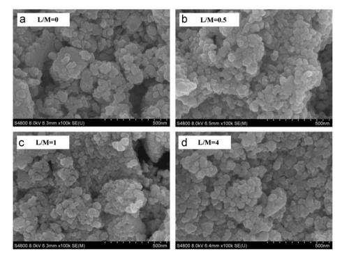
Fig. 5. SEM photographs of the GDC powders with different molar ratios of acrylic acid to metallic ions (L/M) of 0, 0.5, 1 and 4 calcined at 600 °C.
